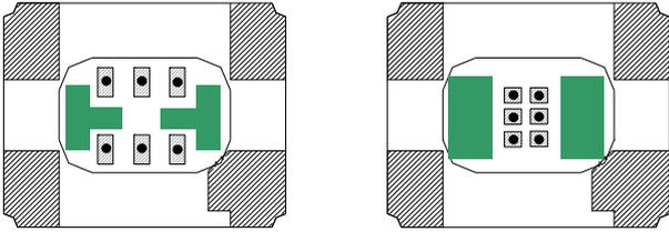
Figure 7. Comparison of the conventional package design (left) and the new design in a 1210 package (right)
