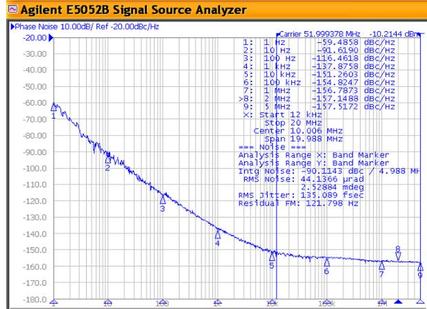
Figure 10. Phase noise measurement of 52 MHz TCXO (1210 size)
