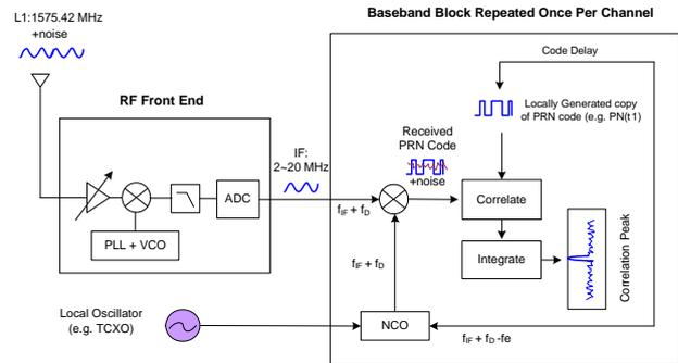
Figure 2. Standard GPS receiver architecture with the RF front end, baseband section and local oscillator
