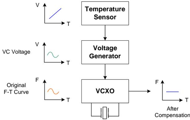
Figure 3. Standard block diagram of analog TCXO
