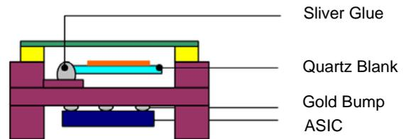
Figure 6. TCXO with H-type package structure
