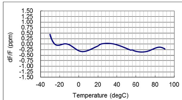
Figure 11. Frequency stability vs. temperature
