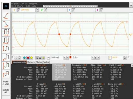
Figure 9. TCXO Clipped-sinewave output with 1.0 V<sub>p-p</sub>
