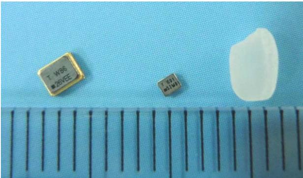
Figure 8. Comparison of the mainstream product in 2520 size (left) and the new product in 1210 size (right)
