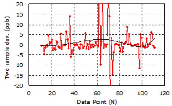
Figure 5. TCXO with improper root Allan variance (rAVAR>5ppb, Tau=1sec)
