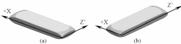
Figure 3. (a) X-elongated and (b) Z'-elongated contour rectangular AT-cut quartz crystal plates
