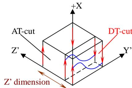
Figure 5. Illustration of AT-cut TS mode and DT-cut face shear mode
