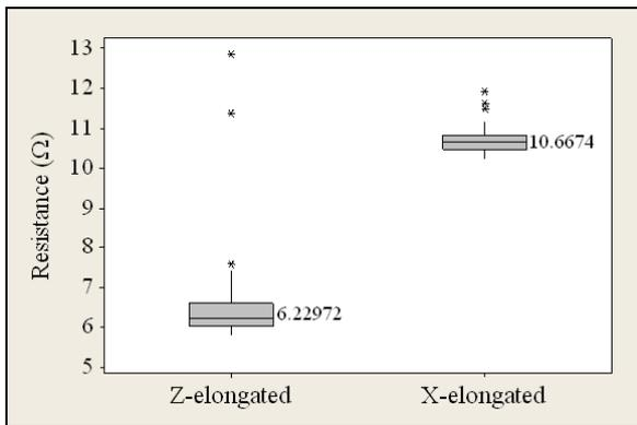
Figure 7. The ESR of Z'- and X-elongated resonator groups with same electrode area
