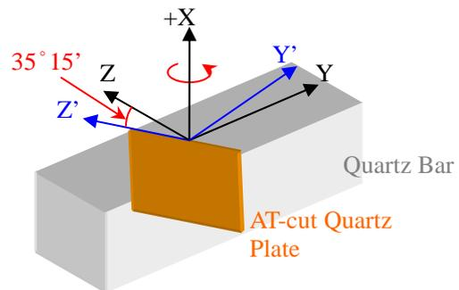
Figure 1. Global coordinate of a quartz bar and the local AT-cut plate coordinate
