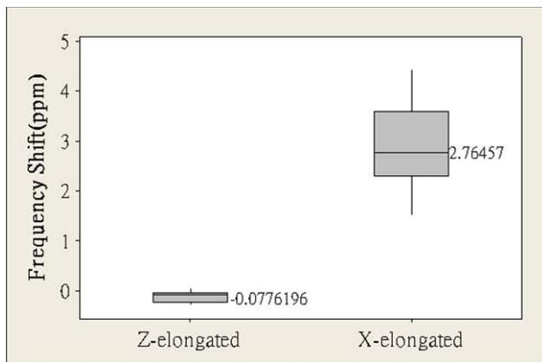
Figure 10. The frequency shift of Z'- and X'-elongated resonator groups due to drop test
