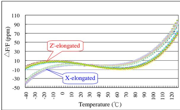
Figure 6. The temperature curves of two resonator groups with same cutting-angle but different length-to-width aspect ratios
