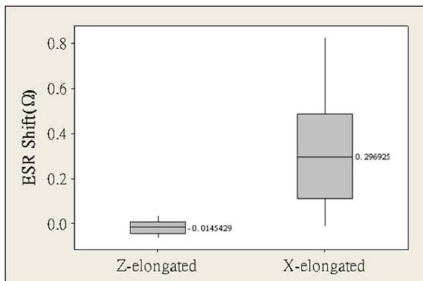
Figure 11. The ESR shift of Z'- and X'-elongated resonator groups due to drop test
