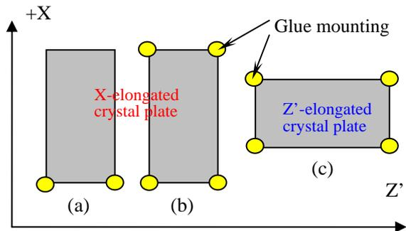
Figure 8. (a) Two corners mounted X-elongated crystal plate
