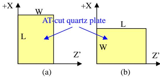
Figure 2. (a) X-elongated and (b) Z'-elongated rectangular AT-cut quartz plates
