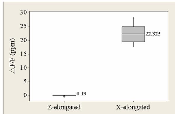
Figure 9. The temperature hysteresis of Z'- and X-elongated resonator groups
