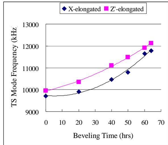
Figure 4. TS mode frequency increasing rate of X- and Z'-elongated crystal plates during beveling
