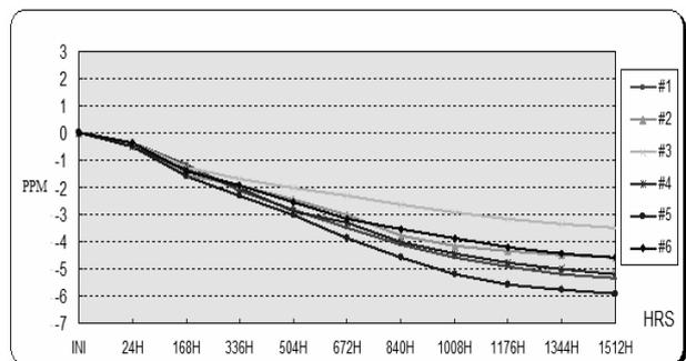
Fig. 7 Accelerated Aging Test at 950  $\mu$ W Dissipation
