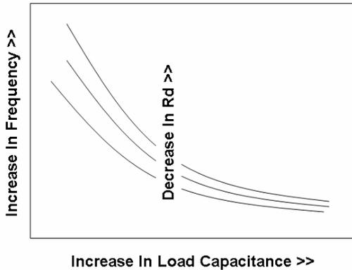
Fig. 3 Frequency vs Load Cap with Varying  $R_d$
