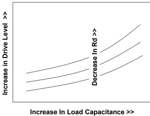
Fig. 4 Drive Level vs Load Cap with Varying  $R_d$
