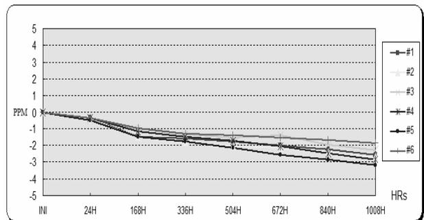
Fig. 6 Accelerated Aging Test at 650  $\mu$ W Dissipation
