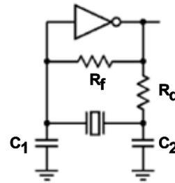
Fig. 2 Typical Pierce Oscillation Circuit
