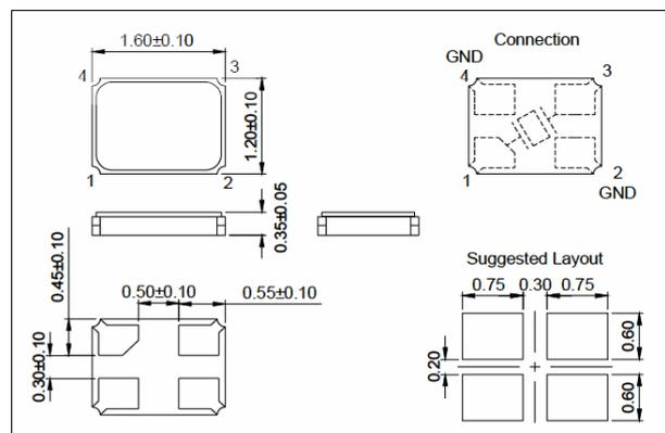
Fig. 1 1.6mmx1.2mm Quartz Crystal from TXC Corporation
