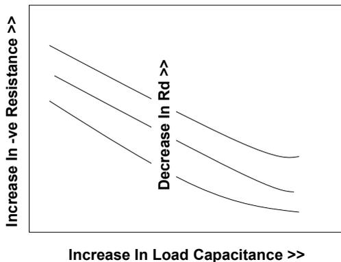
Fig. 5 Negative Resistance vs Load Cap with Varying  $R_d$
